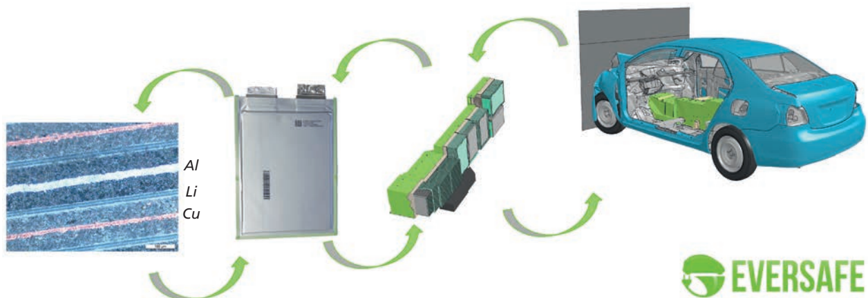
9 Tasks of Fraunhofer EMI in the project EVERSAFE: Starting with cell analysis, the modeling of battery cells and cell materials over vehicle batteries to full car crash simulation under various load case was considered.
