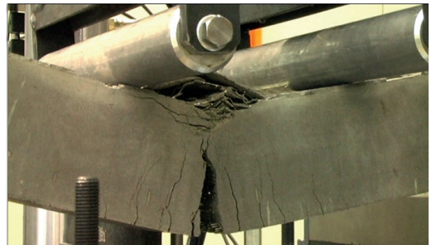
16 DUCON™ element at static tensile test.
