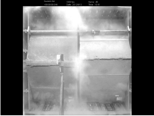
18 Picture sequence of a shock tube experiment on the DUCON™ element at times (from left to right, from top to bottom) t = 0 \text{ ms} , 10 \text{ ms} , 20 \text{ ms} , 30 \text{ ms} , 40 \text{ ms} , 50 \text{ ms} .
