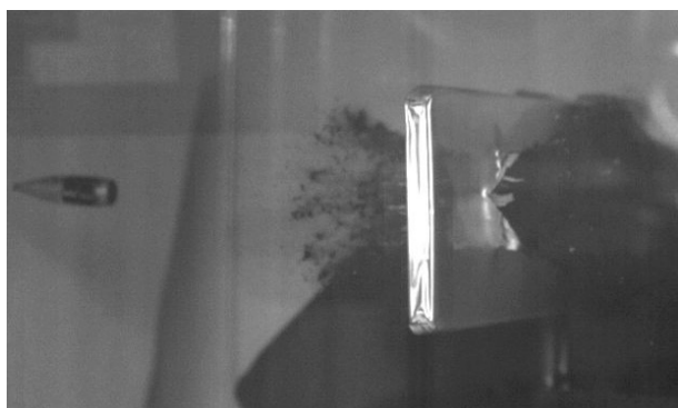
17 High-speed-photographs of the bombardment of charged pouch cells. Left: without backing, right: with steel backing.
